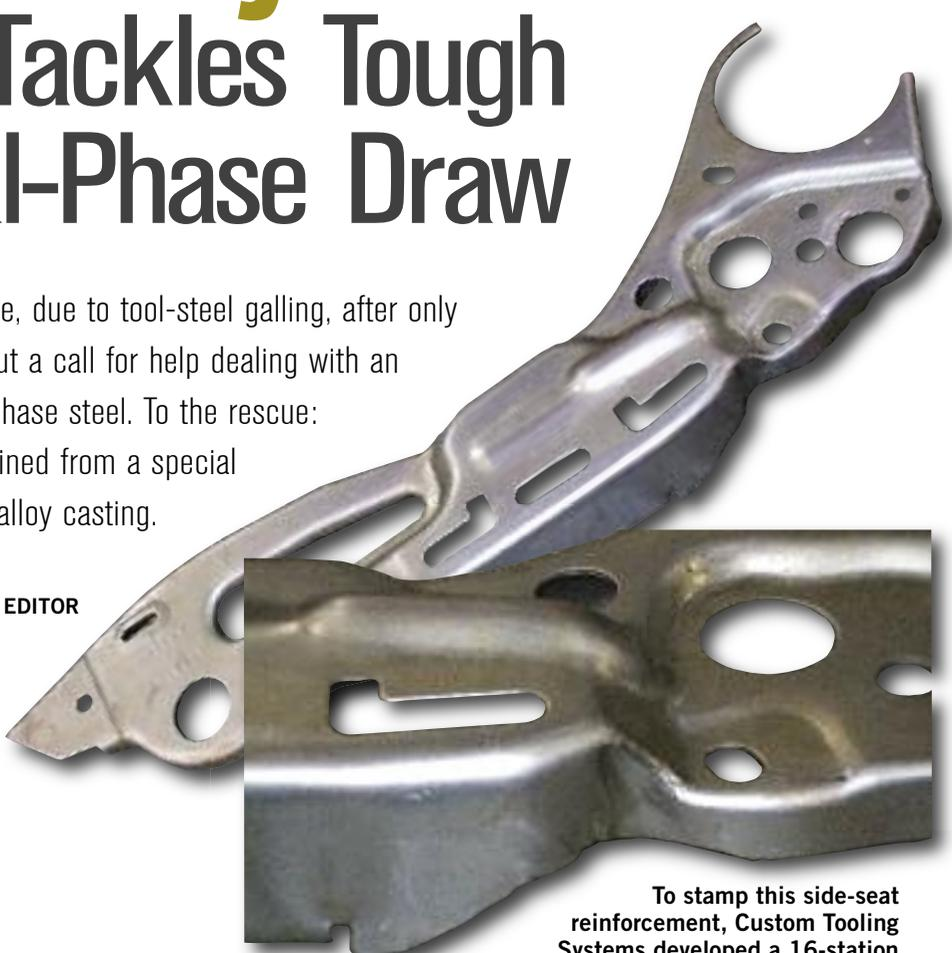
To stamp this side-seat reinforcement, Custom Tooling Systems developed a 16-station progressive die. The part is of 1.5-mm dual-phase steel, which posed significant tooling challenges, particularly in the area where the top surface steps down  $\frac{3}{4}$  in. and then gets flanged 90 deg. For that challenging form station, CTS machined a tool insert of a hardened copper-alloy casting, and to date the tool has made more than 100,000 hits.
